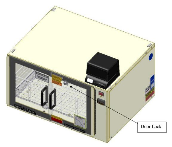
9. When finished, push the shelf back into the HEAT-STACK®, close the doors. The HEAT-STACK® will continue to operate while the doors are open.
